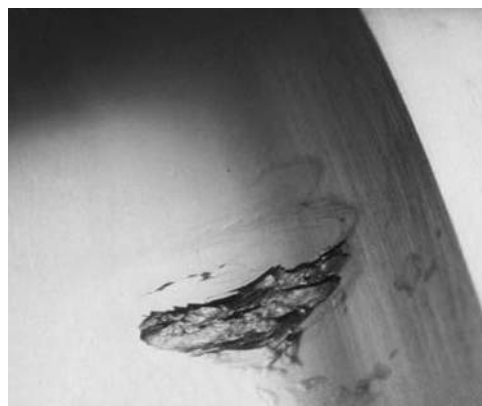
Fig. 5.2 Photo-illustration of fatigue damage on the raceway
